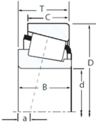
tapered roller bearing 30305 timken bearing
